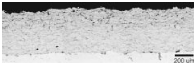
Fig. 4 AL153 coating applied to 1008 steel with the HVOF method
